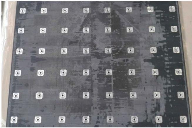
Upper side of the CFC/aluminium foam sliding plate (clamping surface)
