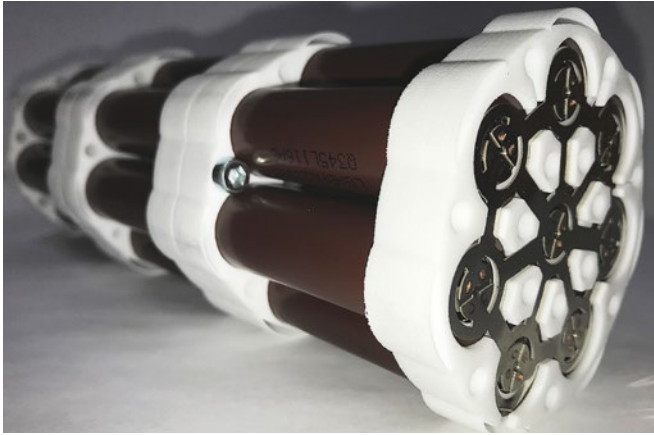
Tubular energy system (TES), which is integrated into the centre tube of the front end of the tricycle in a way that makes it theft-proof.
