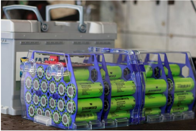
70 Ah lead battery next to 140 Ah lightweight starter battery
