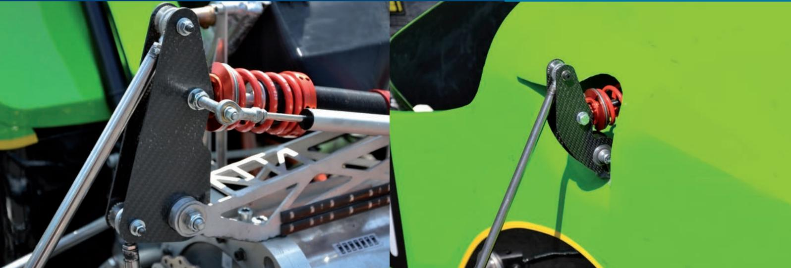
Fibre-reinforced plastic/metal composite for use in vehicle construction
