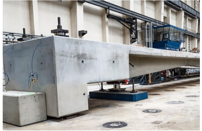
Prototype of a carbon concrete bridge with prestressed CFRP strands
