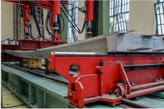
Trapezoidal folded structure made of prestressed carbon concrete during 4-point bending test
