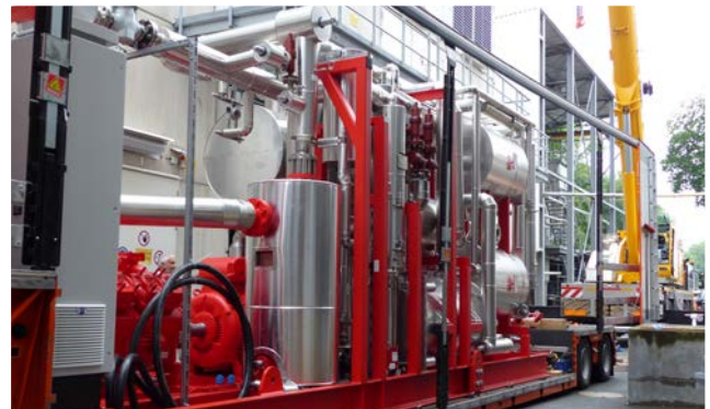
In the HT heat pump project, researchers have developed a compression heat pump with a solution circuit.
