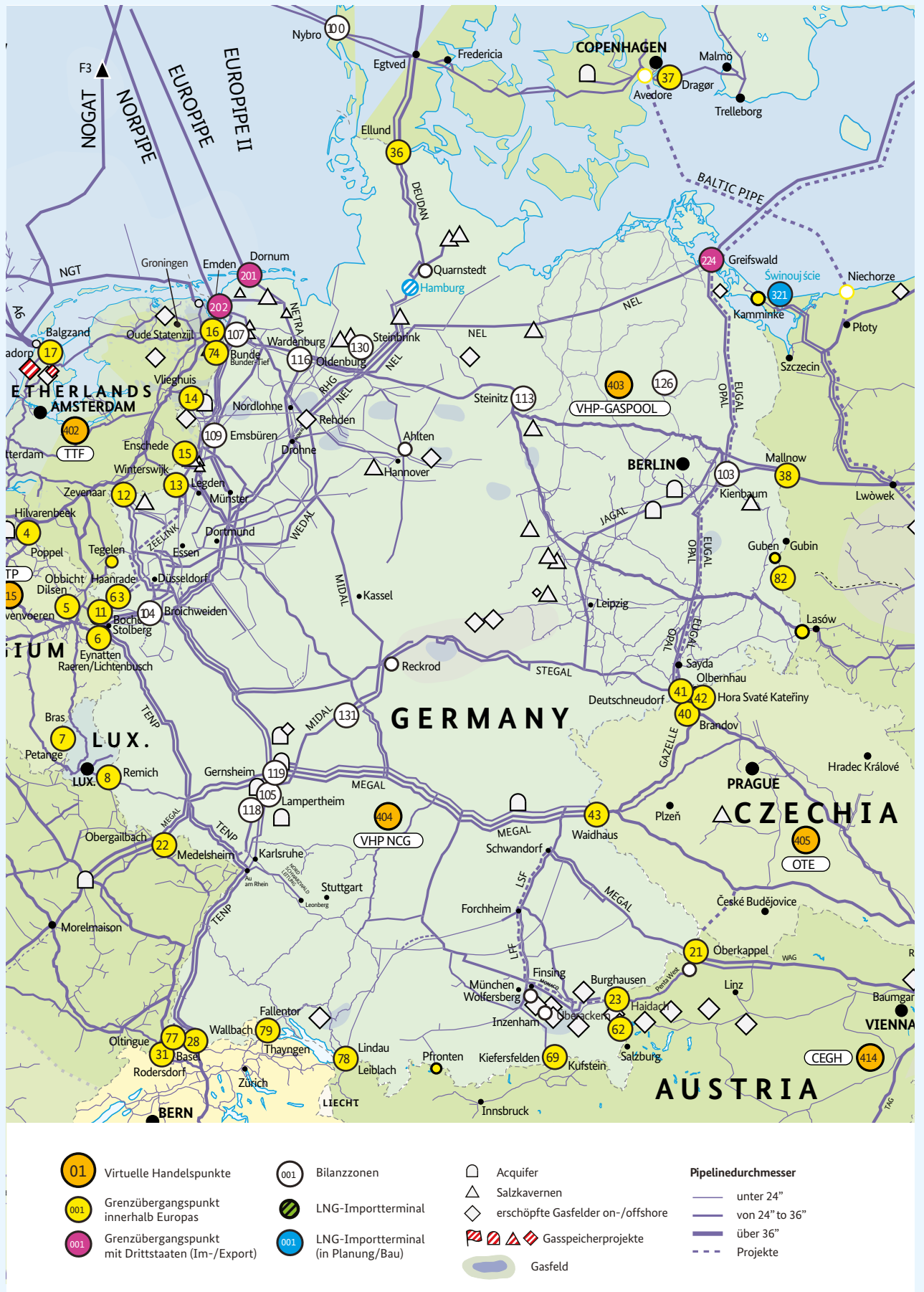
Figure 4: The German long-distance gas grid and its integration in the European transport infrastructure
