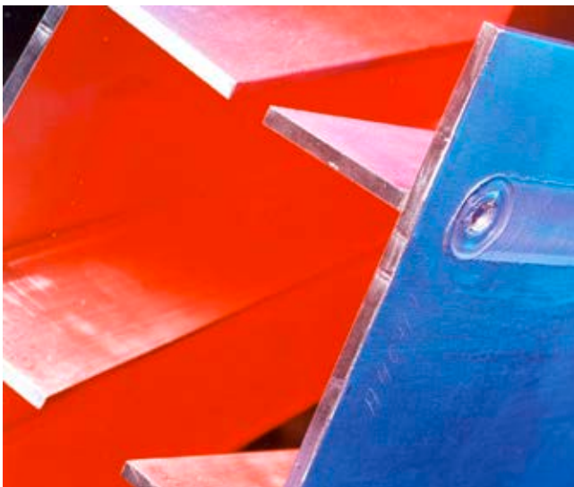
Friction-stir-welded integrated structure for weight reduction.
