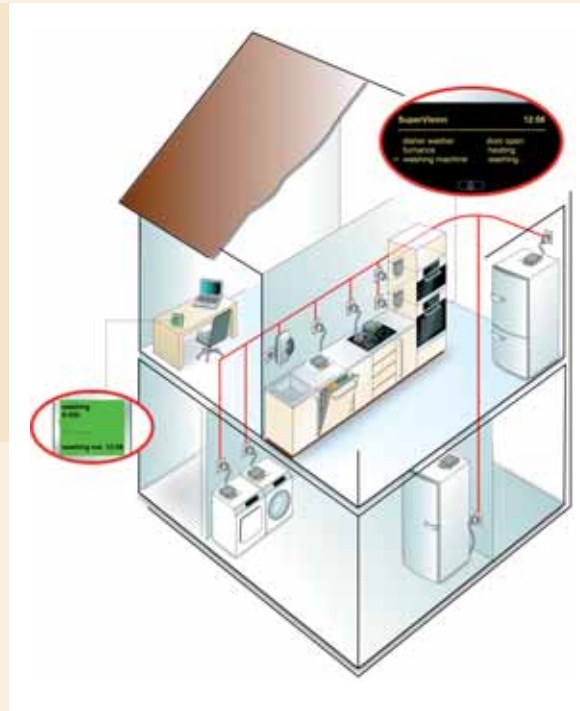
The integrated, networked house allows economical energy management.
