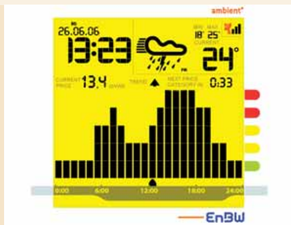
Display unit for previewing the price of electricity.
