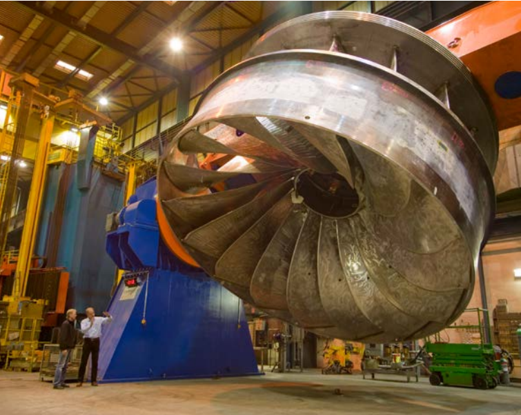
Figure 6: Francis turbine for the Guri hydroelectric power plant in Venezuela
