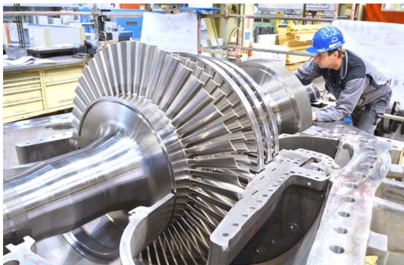
Figure 22: x Process gas expander of a compressed air energy storage system
