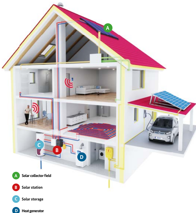
Figure 12: Solar thermal energy system for domestic water heating in a detached house
