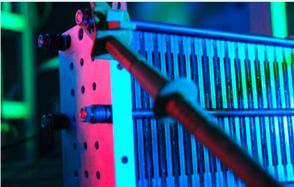
Test of a stack as part of the project to extend the lifespan of PEM fuel cells
