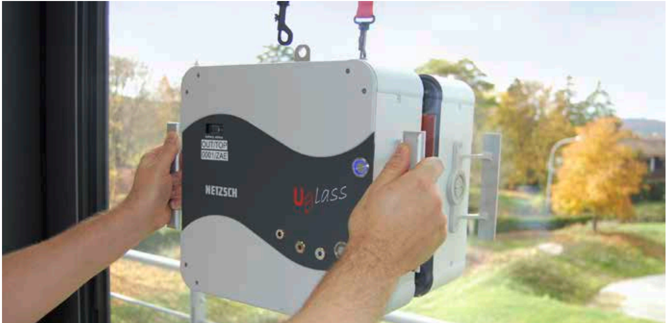
EnOB: The FensterCheck project: Measurement device for determining the thermal quality of glazing
