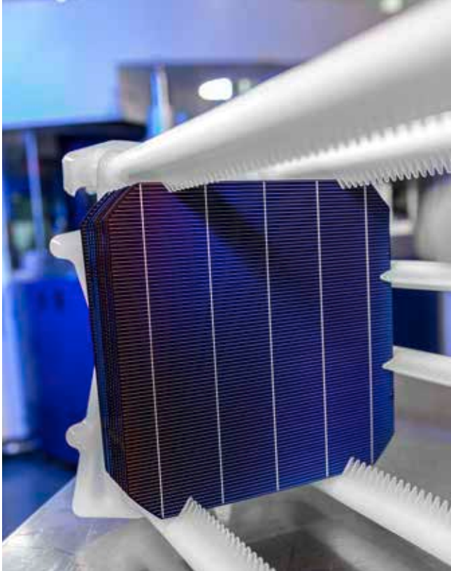
The record-holding PERC solar cell from ISFH with an efficiency level of 21.2 percent
