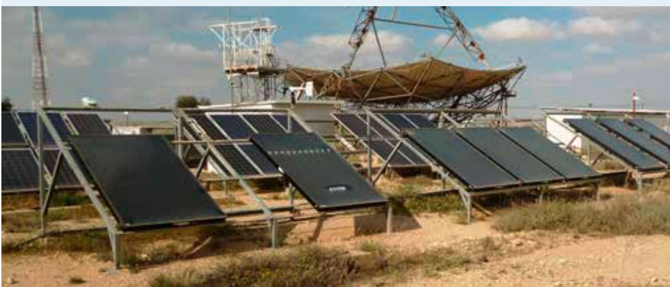
In the Negev desert, scientists from the Fraunhofer ISE are investigating the ageing of solar collectors and components under extreme climatic conditions
