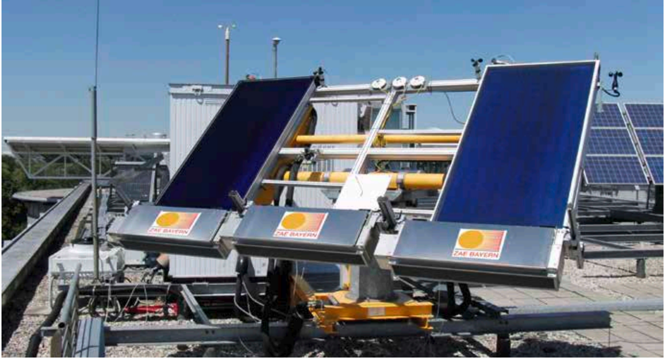
2-axis sun tracker from ZAE Bayern with its first functional models
