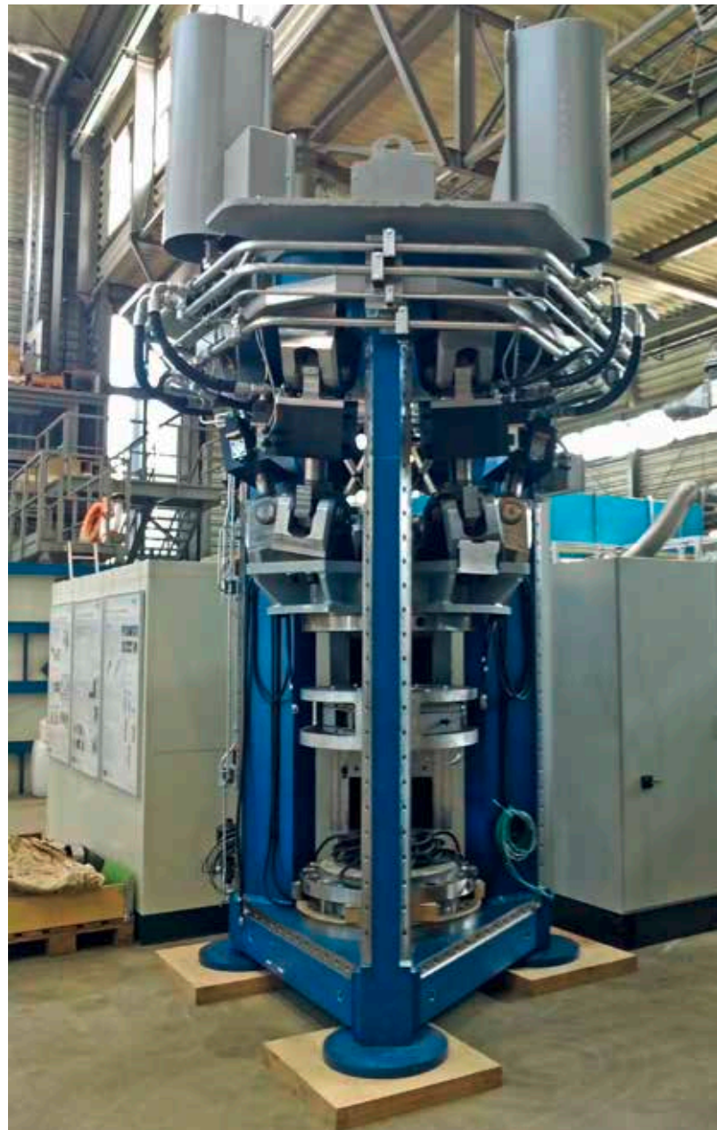
Welding robots for casing pipes
