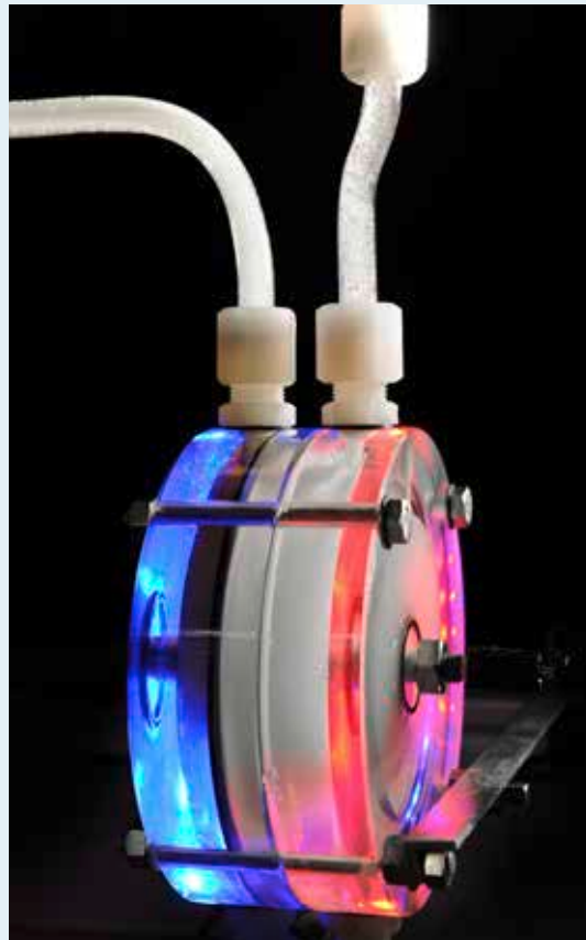
Alkaline electrolyzer stack: The scientists of the project “PlanDelyKaD”, coordinated by the DLR, studied the theoretical conditions for testing an integrated system of “Electricity, hydrogen, large-scale storage and usage” on a scale relevant to the energy industry
