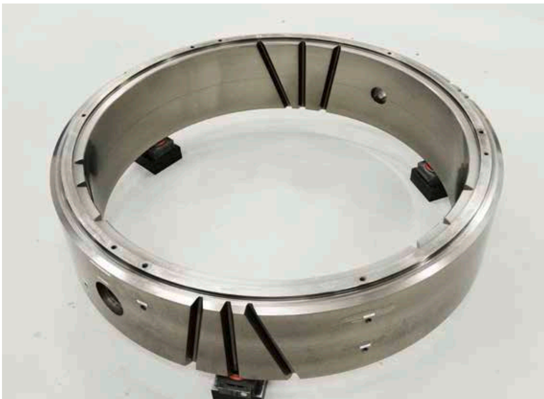
A workpiece-like large gear measurement standard developed by the PTB in the EVeQT project
