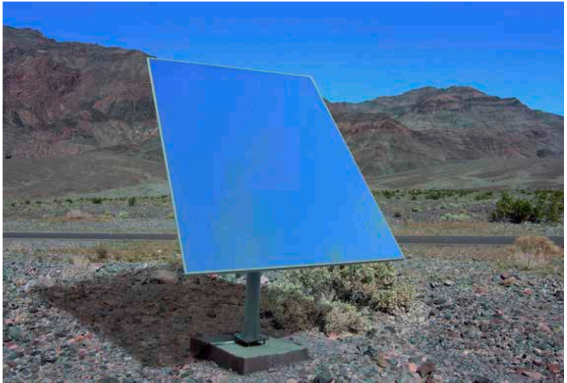
Heliostat from Solar Tower Technologies AG with fixed horizontal axis suspension
